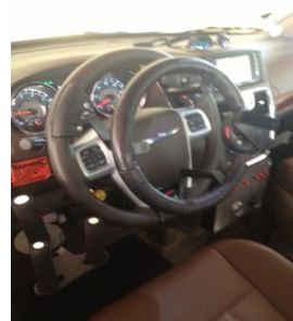
HC Steer and Ext: Push/Rock hand controls with a tri-pin operating handle on the left side. 12" steering wheel extension with a 12" wheel and palm grip steering device. Client is a C7 Tetraplegic w/ transfer ability.
