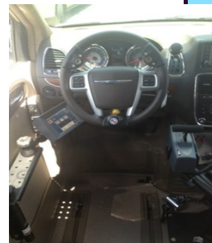
EMC L: Set-up for wheelchair driver with Low Effort Steering w/ spinner knob and electronic gas/brake. Client is a C5 Tetraplegic.
