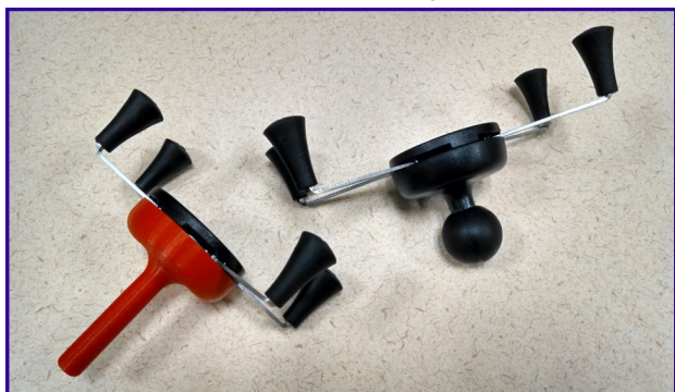
Figure 5—Cellphone mount modification
