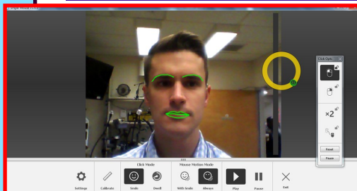
Fig 1. The Smyle Mouse software control screen, from which calibration is initiated and one's settings can be adjusted. The tracking shows the software's ability to recognize a person's eyebrows and mouth
