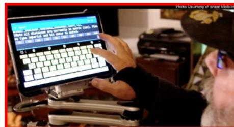
Figure 6. Phil using the Braze Mobility Bluetooth Customization Terminal on his Samsung Galaxy tablet. This feature of the Braze Sentina allows him to customize the distances monitored by the system, the type of feedback provided (visual, auditory, vibratory), and the intensity of the light brightness from the LED display.
