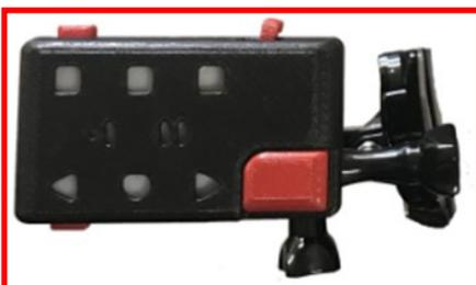
Figure 4. LED display and control panel (front view) that indicates location and proximity of obstacle.
