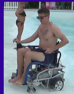
The air-powered Pneuchair wheelchair entering a wave pool (2017)
