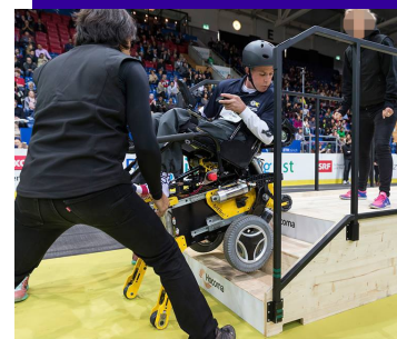
The curb-climbing, seat-leveling MEBot robotic wheelchair competing in the Cybathlon for robotic technology (2016)
